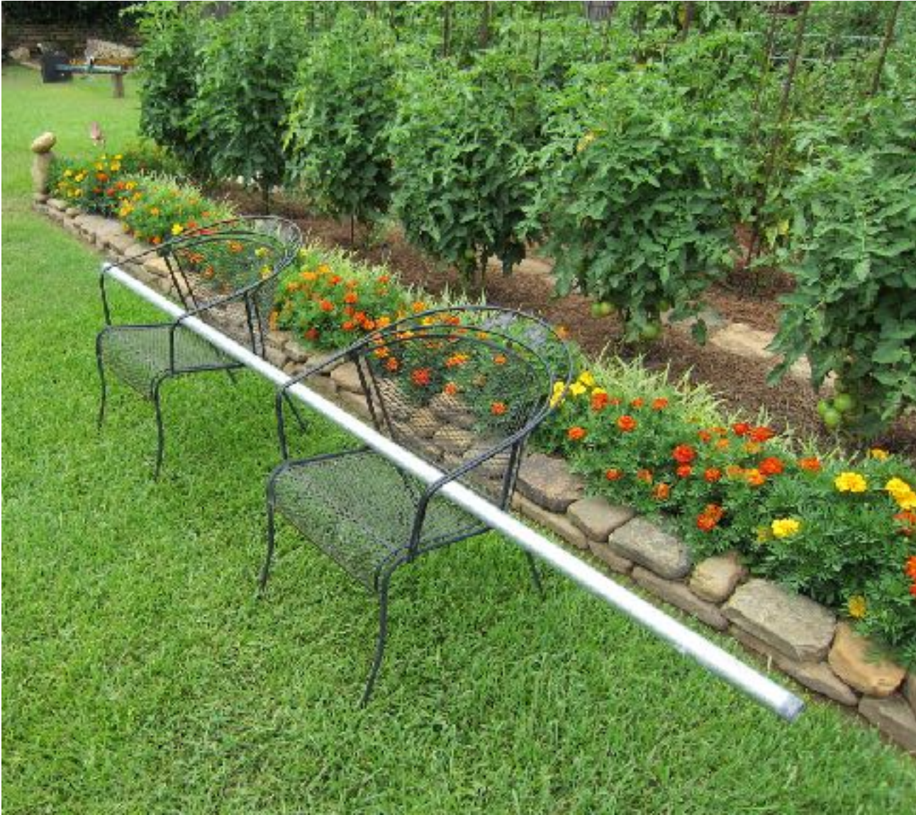
Chairs can be used to hold pipe while marking and drilling.
